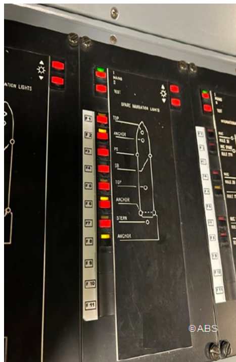
Navigation light and spare anchor light found inoperable
