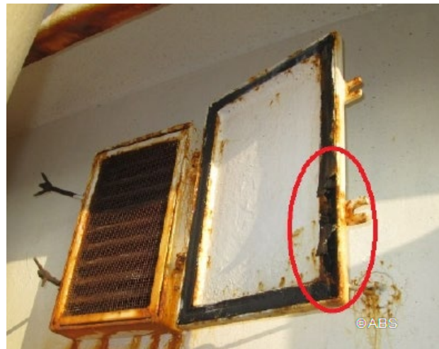
Wall type ventilator – rubber packaging damaged
