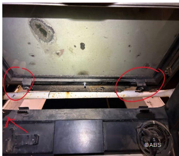
Crane operator cabin, two hinges of emergency exit at lower window broken
