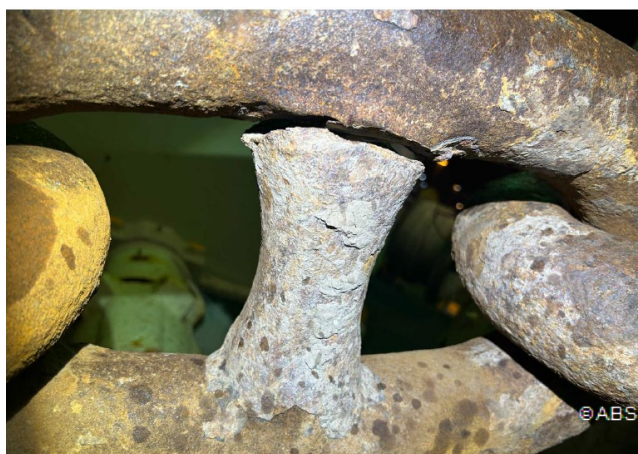
Port anchor chain found with loose stud at multiple links
