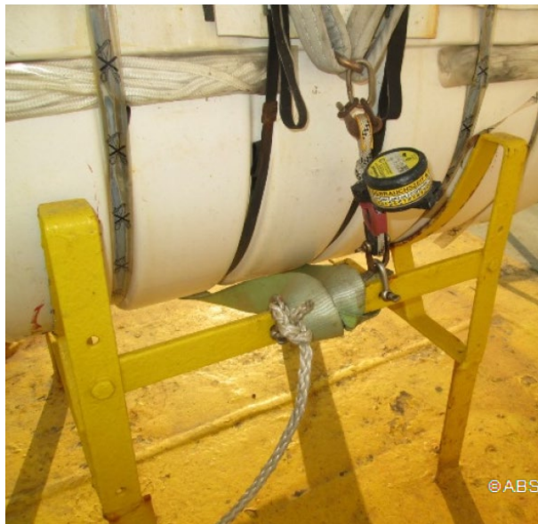
Life raft painter not properly connected
