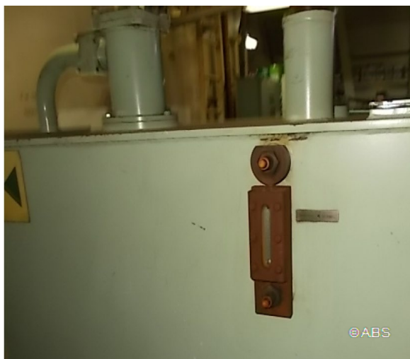
Steering gear system, hydraulic tank level gauge glass showing empty
